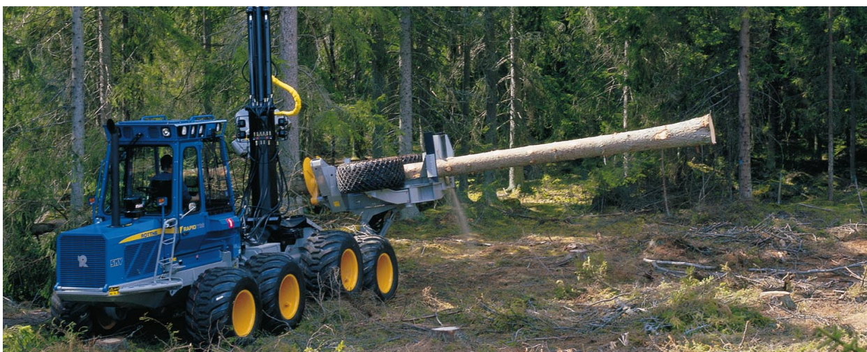
Trelleborg Wheel Systems has developed wide tires for forestry and farming equipment. The tires can be used at extremely low air pressure, which reduces soil compaction and field damage and protects roots near the surface.
