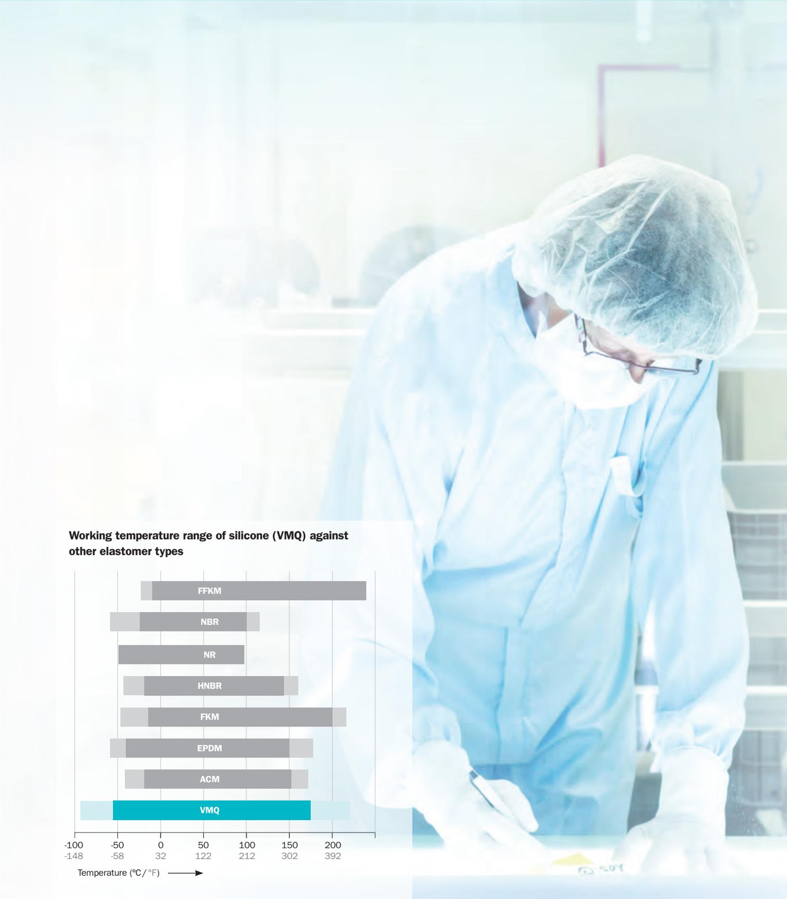
**Working temperature range of silicone (VMQ) against other elastomer types**
