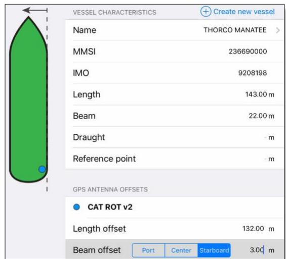
When getting the data from pilot plug of the ship, the dimension and antenna offsets are sometimes wrong. These can be adjusted here to correct for these errors.
