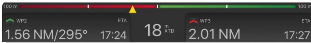
On the left hand side of this panel is the “next waypoint box”. This box displays the ETA distance and bearing to next waypoint. You can tap this box to get a list of waypoints showing the ETA, bearing and distance travelling *directly* towards another waypoint. From this list you can also reverse the route. If you tap on the ETA text in the box you can toggle between ETA and TTG (Time To Go). All calculations of range, bearing, ETA, and XTD are originating from the conning position.
