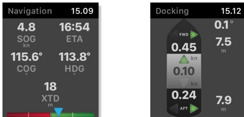
The navigation context shows speed over ground (SOG), heading (HDG), course over ground (COG), cross track distance (XTD) and estimated time of arrival (ETA) or time to next waypoint (TTG). Tap ETA to switch between ETA and TTG.
