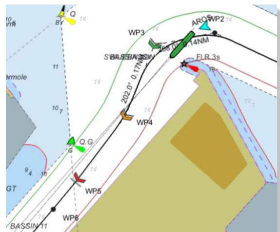
Wheel over points may be added to waypoint indicating when to start turning for the upcoming curve. Long press on the waypoint while editing the route to add the wheel over point distance.
