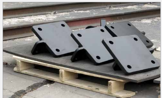
Unloaded chain fixing bracket laying on wooden pellets
