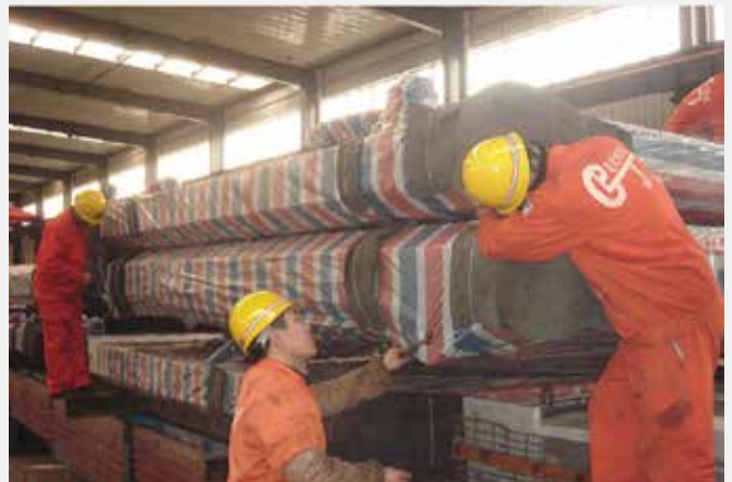
Packaging of stored frontal frame + PE pad assembly
