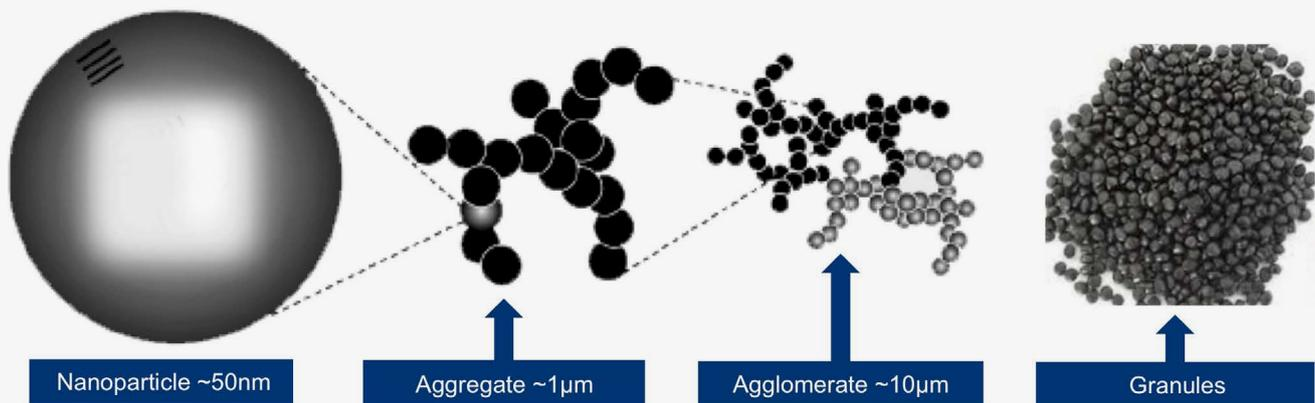
Ideally, carbon black should be broken down into nanoparticles and distributed into the rubber matrix. However, it requires an extremely advanced mixing machine to break it down to aggregate level, the bare minimum to ensure an intimate dispersion within the rubber matrix.
