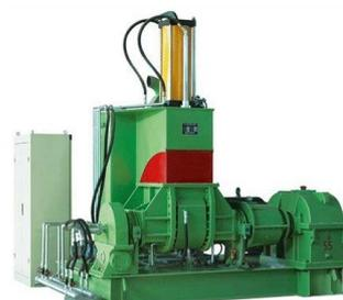
The Internal Mixer is equipped with an automatic ingredient weighing system, which removes the possibility for human error and variation in batch production. The rotors used are also specially designed for the effective tearing and shearing of rubber.
