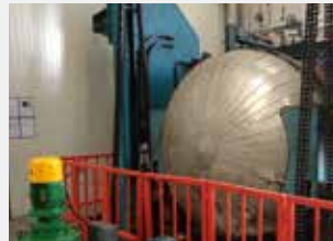
Curing in autoclave
