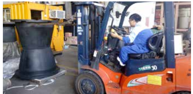
Figure 2 – Fender lifting using forklift
