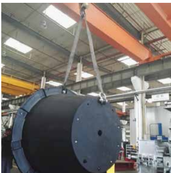
Figure 1 – Fender lifting using crane hook
