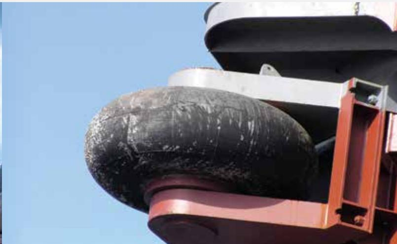
Roller fenders are usually installed to guide ships in restricted spaces like walls of dry docks.
