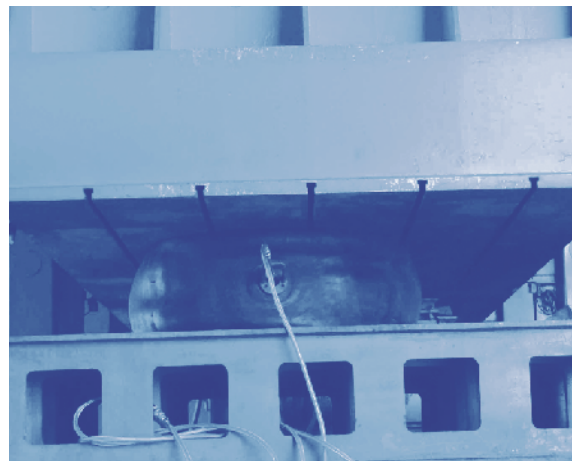
Parallel compression test 60% (PNEUMATIC FENDER SIZE: 1000mm DIAMETER X 1500mm LENGTH)
