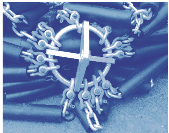
CTN chains connected to the tow ring on a Type I fender
