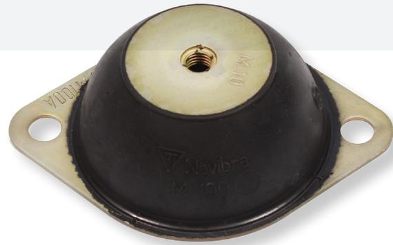
When using M mount together with the height adjuster HA, it is necessary to use a washer. The diameter of the washer must be 20% larger than the diameter of the upper plate (D).
