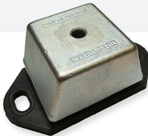
The top metal cover gives protection against oil contamination and the protective finish resists corrosion attack. Two basic designs and different rubber compounds allow loads between 85 and 1070 kg to be accommodated.
