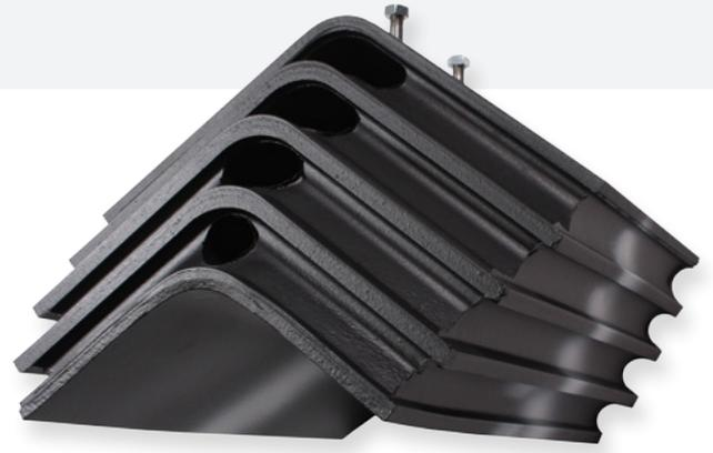
Chevron Springs provide three modes of flexibility for axlebox primary suspensions. The suspension properties are achieved by fitting the springs in a vee formation and with shear and compression compliance within the rubber elements. Improved ride characteristics are provided with the advantages of simplicity, long service life and low maintenance costs.
