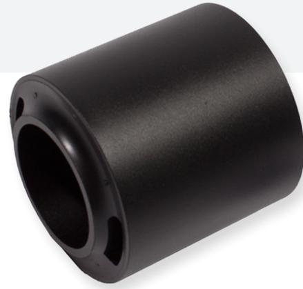
Metalastik UD bush consists of two concentric sleeves with rubber securely bonded between them. Designed to accommodate torsional movements, axial and radial loads. The rubber is pre-stressed to give maximum dynamic strength and durability.
