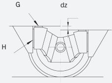
The vertical deflection (dz) may vary due to creep, Joule effect and stiffness tolerances. Shims (G) should be included for height adjustment. Shims (H) are sometimes necessary for accurate alignment of axles.
