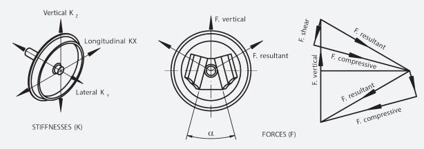
The three modes of flexibility for axlebox suspension are shown here. Springs are fitted inclined at an angle to the vertical axis, loading the rubber layers in shear and compression.
