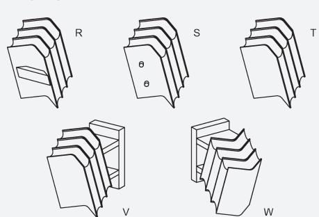
Springs can be supplied with alternative methods of location as shown in the diagram, namely with cross bar (R), dowel pins (S), or edge location (T). Location on the bogie frame is normally on the plate edge. Springs can be supplied with brackets for direct and easy fitting to the bogie frame (ref . figs V & W)
