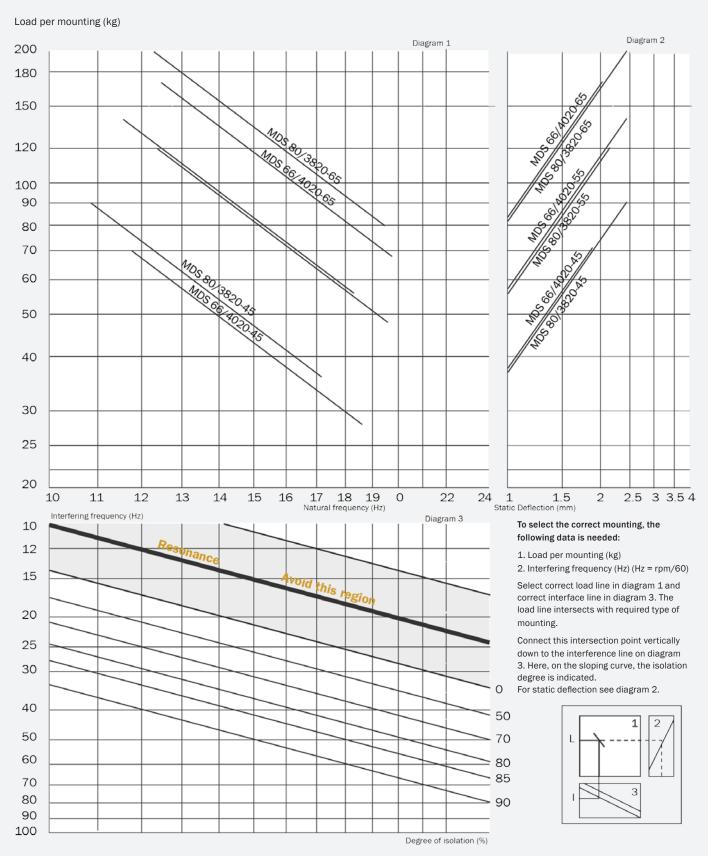
Note: The natural frequencies and degrees of isolation are based on dynamic characteristics of the mounting
