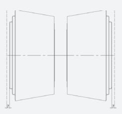
The conical bearings shall be mounted in pairs and preloaded axial roughly 7 mm each.
