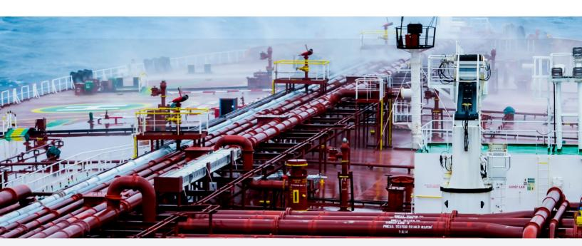
Pipeline systems are exposed to temperature variations, chemicals, setting in foundations, forces, and deformations causing movement and/or stress in the system. To ensure flawless operation of the system it is necessary to insert flexible parts to absorb the moments preventing structural damage.
